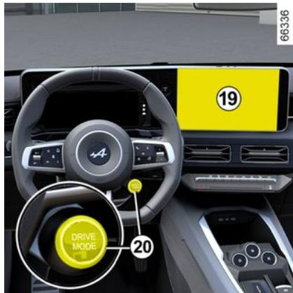
From the DRIVE MODE menu which can be accessed from the multimedia screen **19** or by pressing the switch **20**, you can activate Save mode which affects the heating level and reduces the vehicle's fuel consumption.
