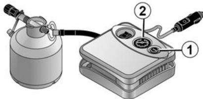
In the event of a puncture, use the kit located underneath the luggage compartment carpet.
