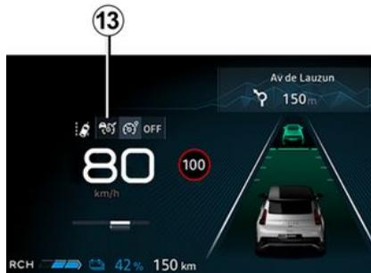
Press switch **3** to select the adaptive cruise control at **13**. The warning light **9** appears in grey. The "Adaptive Cruise Control ready: SET to activate" message appears on the instrument panel accompanied by dashes to indicate that the cruise control function is in operation and waiting to store a cruising speed.
