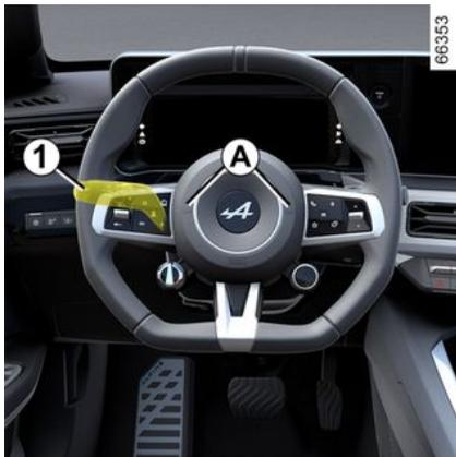
Press the steering wheel boss **A** to sound the horn.
