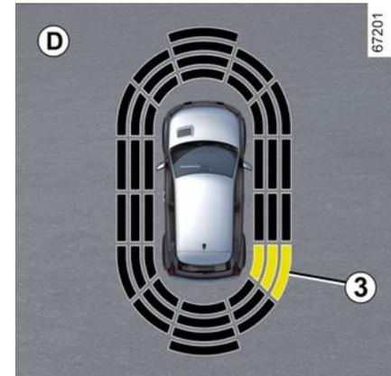
Depending on the direction of the wheels, the system determines the vehicle trajectory and notifies the driver if there is a risk or not of a collision with an obstacle **3** to the side of the vehicle.
