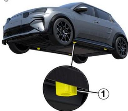
Your vehicle is equipped with four dedicated lifting points **1** located underneath the vehicle.
