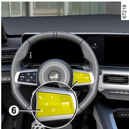
Depending on the vehicle, by pressing the steering wheel control **6**, you can activate the heated seats according to the stored user settings that you have previously defined.
