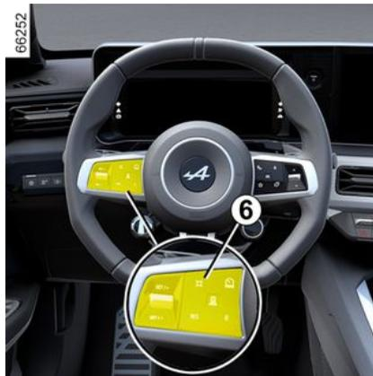
To adapt the speed limiter, cruise control or adaptive cruise control setpoint to the detected speed limit, press the 6 switch.
