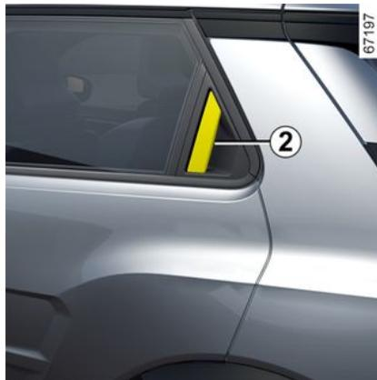
With the doors unlocked or the card on you, hold the handle **2** and pull it towards you.
