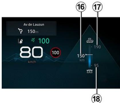
High **17**: visibility of range in optimal conditions (e.g. driving on A-roads or dual carriageways with little use of thermal comfort).
