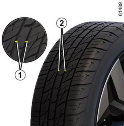
The tyres must be in good condition and the tread form must have sufficient depth; tyres approved by our Technical Department have wear warning strips **1** which are **indicators moulded into the tread at several points**.
