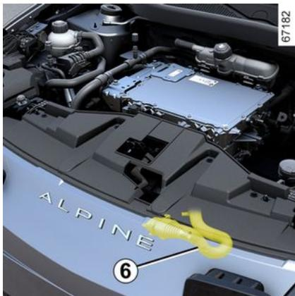
The "400 V" electrical circuit can be recognised by the orange wiring **6** and components bearing the ⚡ symbol.
