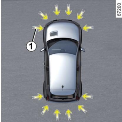
As indicated by the arrows **1**, the ultrasonic detectors installed in the vehicle bumpers help to find accessible parking spaces and assist the parking manoeuvre.
