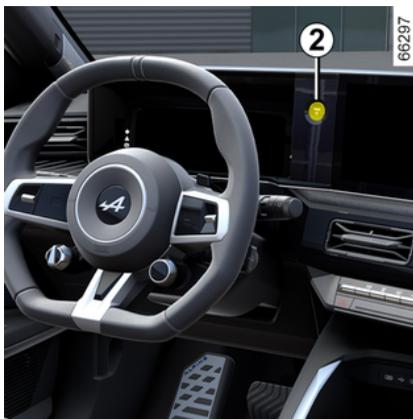
If the smartphone is no longer in the passenger compartment when you try to switch the engine off, a message is displayed on the instrument panel: press and hold the engine start/stop button **2** for more than two seconds.
