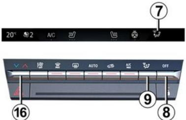
Press on **9** once or repeatedly to adjust the air distribution. The selected air distribution setting **7** is displayed
