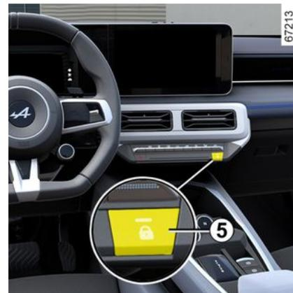
The switch **5** simultaneously controls the doors and the luggage compartment door.
