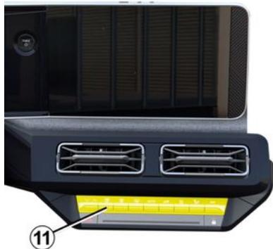
To control the air flow from the air vents **1**, **4** and **6** press or raise the control **11** to the level desired.
