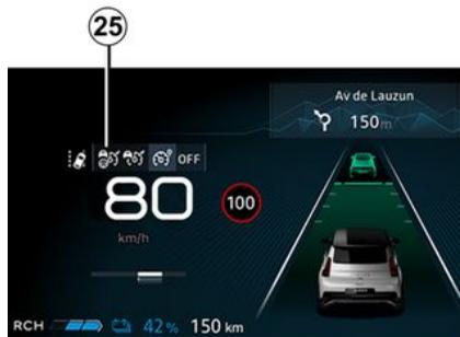
To activate the function, press the switch **9** as many times as required to start it at 25.
