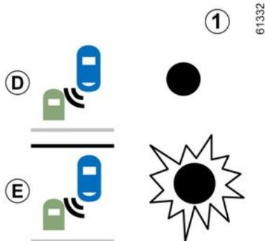
First warning: **direction indicator not activated**, the warning light **1** indicates that a vehicle is detected in the blind spot and/or that a vehicle is rapidly approaching from the rear in an adjacent lane.
