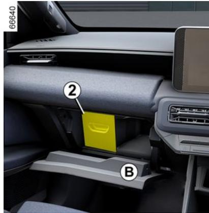
The fuses can be accessed behind the glovebox in the passenger compartment **B**. Open the glovebox using the opening button.
