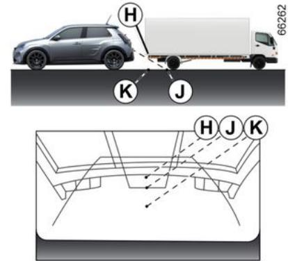
Position **H** seems further than position **J** on the screen. However, position **H** is at the same distance as position **K**.
