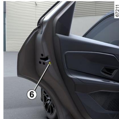
To make it impossible for the rear doors to be opened from the inside, lower the lever **6** and check from the inside that the doors are securely locked.
