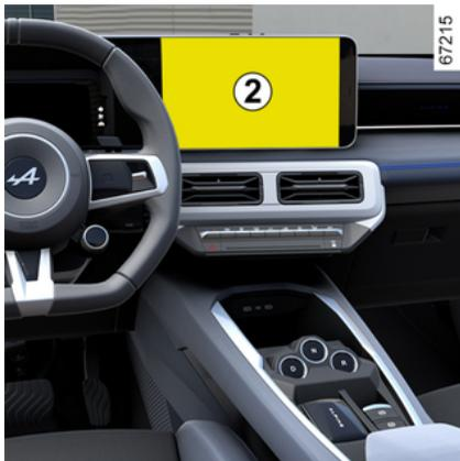
From the multimedia screen **2**, when reverse gear is engaged, press the "Settings" button to add or remove guide lines and to adjust the camera image settings (brightness, contrast, etc.).
