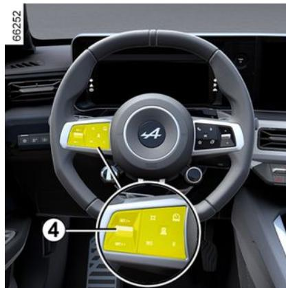
You can change the limit speed by repeatedly pressing or by pressing and holding on control **4**:
