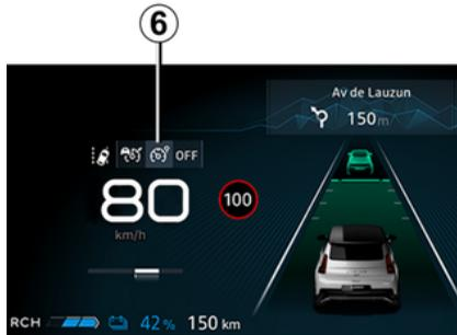
**i** To exit the driving assistance, press switch **1** as many times as necessary until you reach OFF. The "Driving Assistance deactivated" message appears on the instrument panel. In this case, the next time the engine is started, the "Speed limiter" function will be activated and waiting for a speed limit to be stored.
