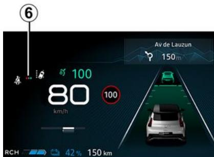
With the doors closed, the graphic **6** is displayed on the instrument panel for approximately 60 seconds when the vehicle ignition is switched on. This informs the driver of the fastening status of each of the front seat belts every time:
