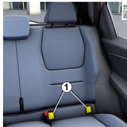
The two rings **1** are located between the seatback and the seat base and
