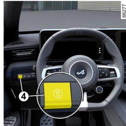
The sound alert can be deactivated or activated using "Custom" mode in the "My Safety" function ➔ **184**.
