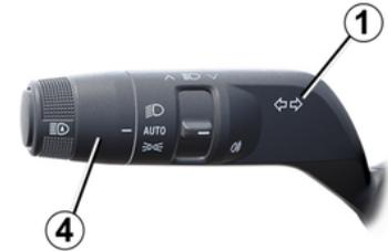
The lights will go out automatically when the driver's door is opened or the vehicle is locked, or one minute after the engine is switched off.
