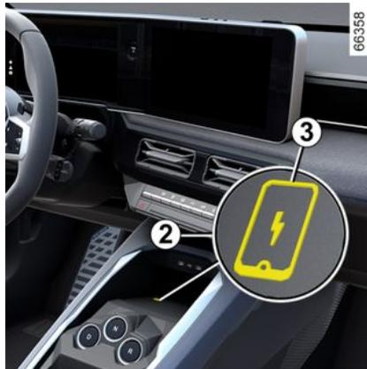
Depending on the vehicle, the 3 symbol indicates that area 2 can be used to charge your phone without using a charging cable.
