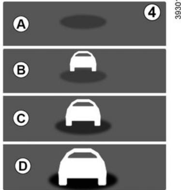
With the function activated, the indicator light **4** is displayed on the instrument panel and informs the driver of the distance between their vehicle and the vehicle in front.
