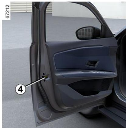
With the door open, turn the screw **4** (using the end of the key) and close the door.
