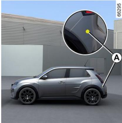
Using information from the radars installed on each side of the rear bumper (zone **A**), the system warns the driver when another vehicle appears in the detection zone **B**.
