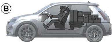
– the front seatbacks with the rear seatbacks folded down, as is the case for maximum loads (example **B**).
