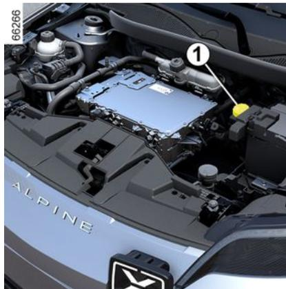
The level should be read with the engine switched off and on level ground. This should be checked frequently, and immediately if you notice even the slightest loss in braking efficiency.
