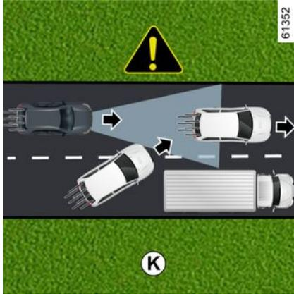
The system detects only vehicles (cars, trucks, motorbikes) that are moving in the same direction as your vehicle.
