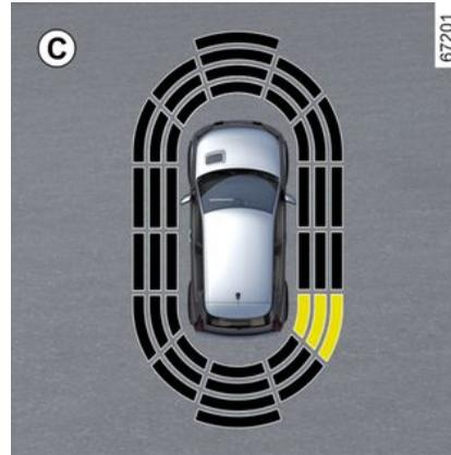
Most objects located less near the front, rear and sides of the vehicle are detected.
