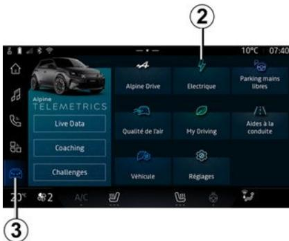
With the vehicle stationary and the engine running, from the "Vehicle" world **3** on the multimedia screen **1**, press the "Electric" menu **2** then the "Charge & Climate" tab to set up charging for your vehicle.
