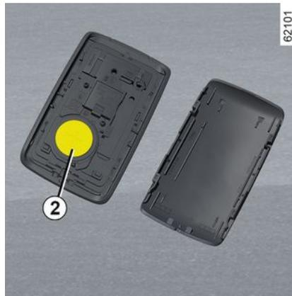
To refit, proceed in the reverse order then press one of the buttons on the card four times while you are near the vehicle: the next time the vehicle is started, the message will disappear.
