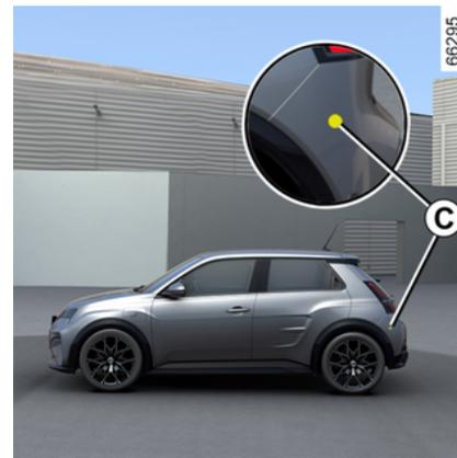
Ensure that zone **C** around the radars on each side of the rear bumper is not obstructed (by dirt, mud, snow, etc.). If a radar is obscured, the "Side radars no visibility" message will appear on the instrument panel. Clean the area where the sensors are located.
