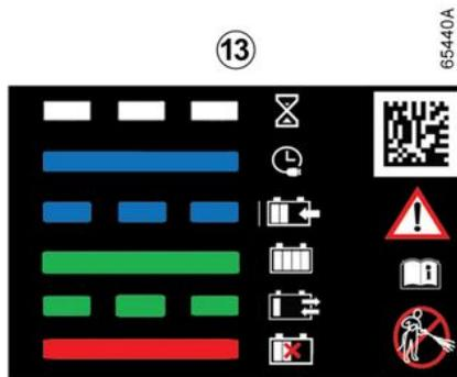
The label **13** located on the charging flap **8** details the charging operation according to the status of the indicator light **9**:
