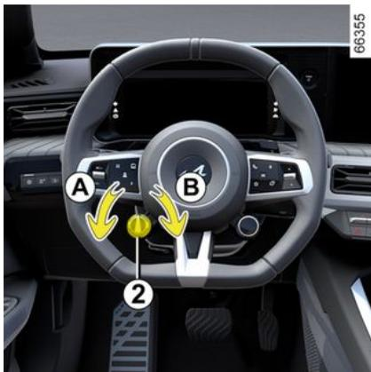
The touch control **2** can be used to change the regenerative braking level:
