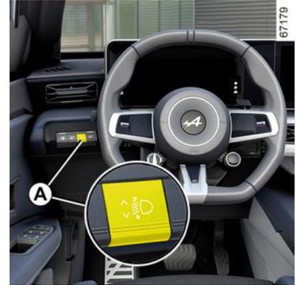
the switch **A** can be used to adjust the height of headlight beams according to the load.
