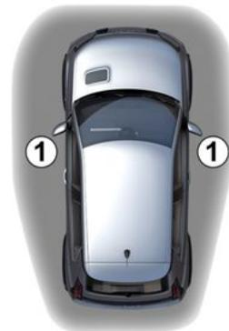
If you are holding the card and in the access zone **1** the vehicle will be unlocked.
