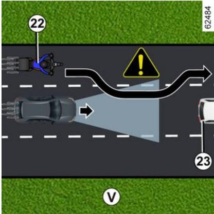
If your vehicle is overtaken by another vehicle driving at high speed **22** (motorcycle, car, etc.) and the vehicle is temporarily positioned between your vehicle and the vehicle in front **23**, **the system may trigger undue acceleration, slowing or braking.**
