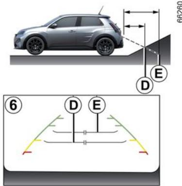
The fixed guidelines **6** show the distances as closer than they actually are. The objects shown on the screen are actually further away on the slope. For example, if the screen displays an object at **D**, the actual distance of the object is at **E**.
