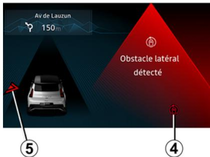
When driving at a speed between approximately 43 mph (70 km/h) and 68 mph (110 km/h), if there is a risk of collision with a vehicle coming from the opposite direction in an adjacent lane and within the detection zone **C**, without the direction indicator having been activated, the system:
