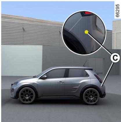
Ensure that zone **C** around the radars on each side of the rear bumper is not obstructed (by dirt, mud, snow, etc.).
