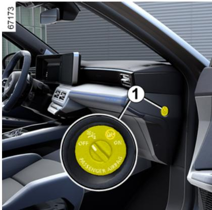
You should reactivate the airbag as soon as you remove the child seat from the front passenger seat to ensure the protection of the front passenger in the event of an impact.
