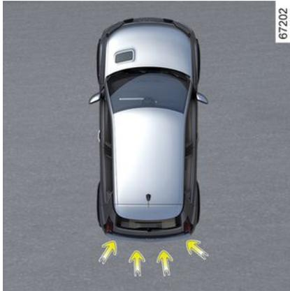
In addition to the "Parking assistance" → 258 function and using information from the four central sensors located at the rear of the vehicle, the system detects fixed obstacles located behind your vehicle. If there is a significant risk of collision, the system automatically causes the vehicle to brake.
