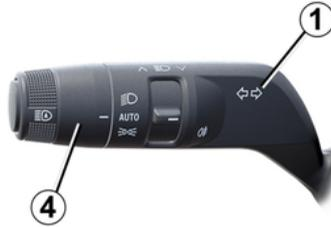
This function enables you to briefly switch on the side lights and dipped beam headlights (e.g. to provide light when opening a gate).
