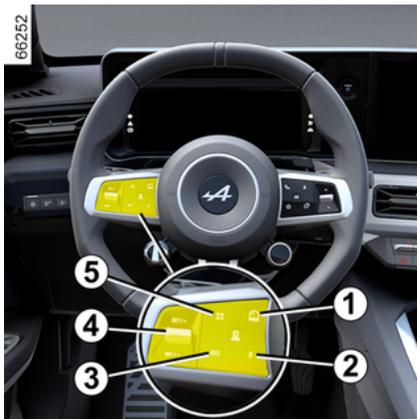
**1.** Switch for selecting/deselecting the driving aids, depending on the vehicle:
