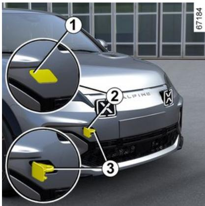
Press the upper section of the flap **1** to tilt it.
