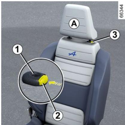
Pull the headrest upwards to the desired height. Check that it is correctly locked.
