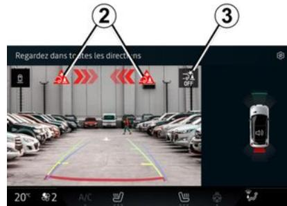
If the vehicle is fitted with a towbar recognised by the system and a trailer has been connected, active emergency braking in reverse gear is automatically deactivated and the following message is displayed on the instrument panel: "Trailer: parking sensors unavailable", accompanied by the warning light **3** on the multimedia screen.
