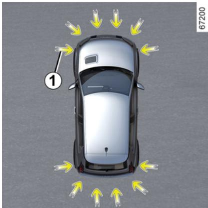
Ultrasonic sensors, indicated by arrows **1**, are fitted in the bumpers to detect obstacles near the vehicle.
