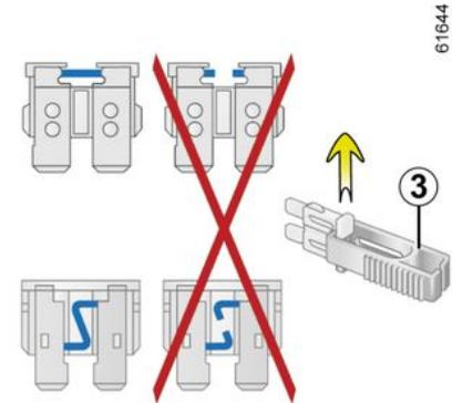
Remove the fuse using the clamp **3** located on the fuse panel.
