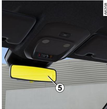
The rear view mirror automatically darkens when you are being followed by a vehicle using main beam headlights or in very bright lighting.
