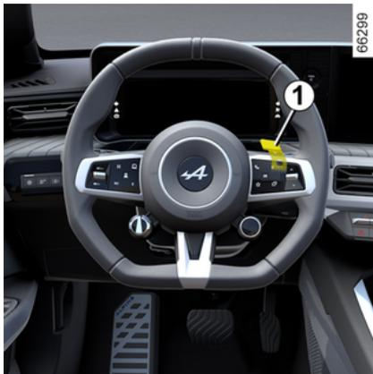
When you press the "OV" button **1** on the steering wheel, the engine delivers the maximum performance, instantly increasing the vehicle's acceleration.
