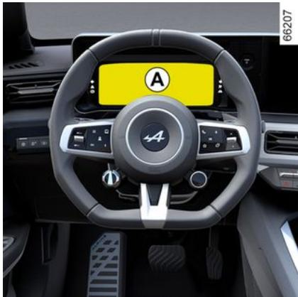
**Instrument panel A:** this lights up when the driver's door is opened. To adjust the dashboard brightness, refer to the multimedia instructions.
