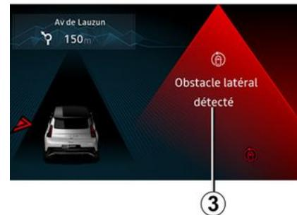
When the detected object is very close, a beep will sound, along with the **3** "Lateral obstacle detected" warning message on the instrument panel.
