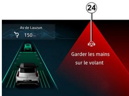
When the "Lane Centring" function no longer detects your hands on the steering wheel, several warning levels will be triggered:
