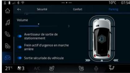
To activate or deactivate the function via the multimedia screen **1**, select the "Vehicle" world, then "Driving assistance", then "Parking". Activate the "Active emergency braking in reverse gear".
