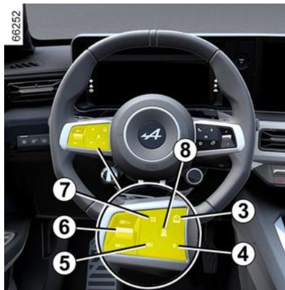
**3.** Switch for selecting/deselecting the driving aids, depending on the vehicle:
