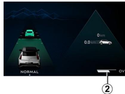
At any time, you can check if the function is available by consulting the remaining range on the "OV" gauge **2** displayed on the instrument panel.
