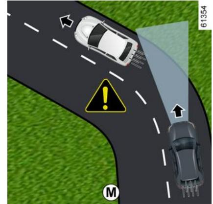
When entering a corner or bend, the radar and/or camera may be temporarily unable to detect the vehicle in front (example **M**).
