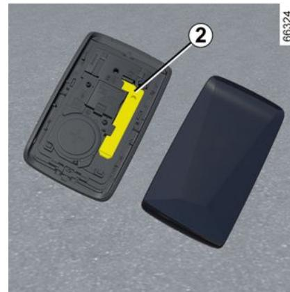
Slide the rear casing 1 downwards while pressing on area A.
