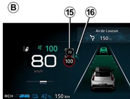
The letter "A" **16** is displayed on the instrument panel to confirm the activation of the cruise control with anticipated speed limit sign recognition.
