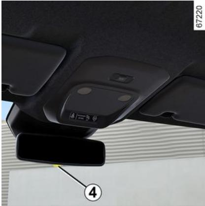
When driving at night, to avoid being dazzled by the headlights of the vehicle behind, shift the small lever **4** located behind the rear view mirror.
