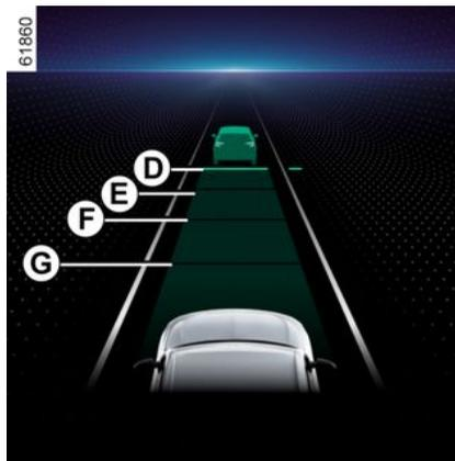
The horizontal distance gauge on the instrument panel indicates the various available safe distances:
