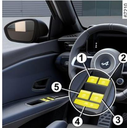
Briefly press or pull a window switch as far as it will go: the window will be fully raised or lowered. Pressing the switch again stops the window moving.
