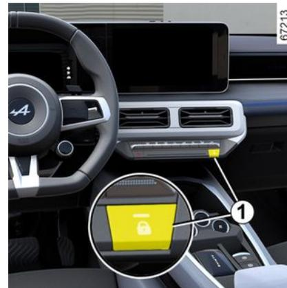
After the vehicle is started, the system automatically locks the doors when you reach approximately 6 mph (10 km/h).
