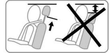
**When the headrest is set at the lowest position, this is for storage only:** it should not be in this position when the seat is occupied.
