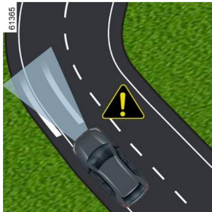
In the case of a sharp bend, and depending on the vehicle speed, the function's side retaining capacities will be limited and require the driver to carry out immediate action on the steering wheel so that the vehicle remains in the lane.
