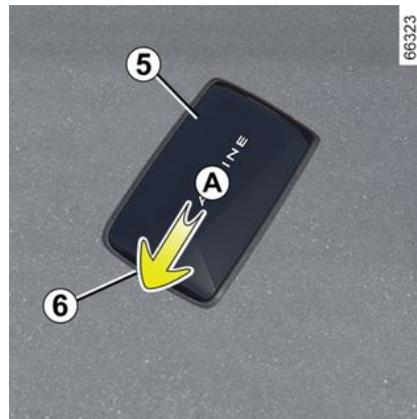
Slide the rear casing **5** downwards while pressing on area **A**.
