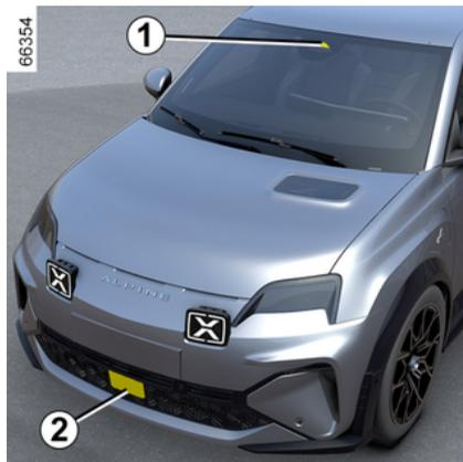
Using information from the camera **1** and the radar **2**, the system determines the distance between your vehicle:
