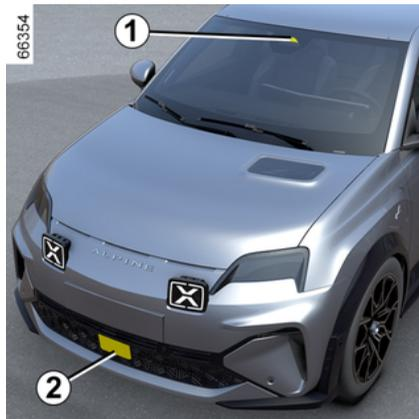
Using the information from the radar **2** and camera **1**, this function informs the driver of the time interval between their vehicle and the vehicle in front so that a safe stopping distance between the two vehicles can be maintained.
