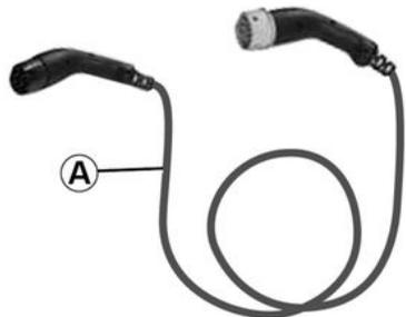
This lead is specific to your vehicle and designed for connecting to wall sockets or public terminals to enable standard charging of the traction battery.
