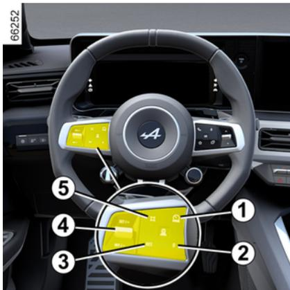
The speed limiter function is suspended when you press switch **2** (0).
