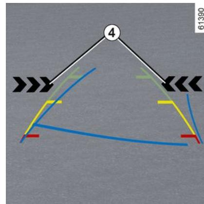
The warning lights **4** on the multimedia screen indicate the side on which the approaching vehicle has been detected.
