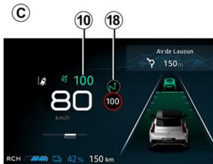
Using the camera, the "Road sign detection" function → 217 and the maps, the system can anticipate and manage the automatic adaptation of the cruising speed **10** when the vehicle approaches a roundabout or a bend.
