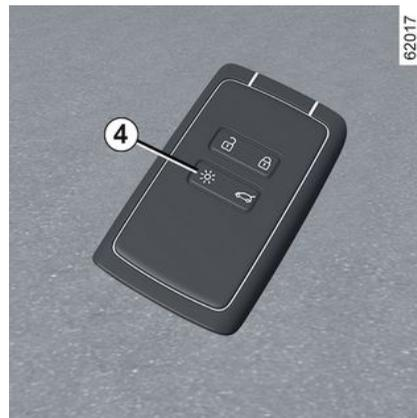
Press button 4 to switch on the dipped beam headlights and the exterior lighting for approximately 20 seconds. This can be used, for example, to identify the vehicle from a distance when parked in a car park. Press and hold button 4 for approximately two seconds to switch on the exterior lighting and emit a sound.
