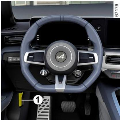
To open, pull the handle **1** located on the left-hand side of the dashboard.
