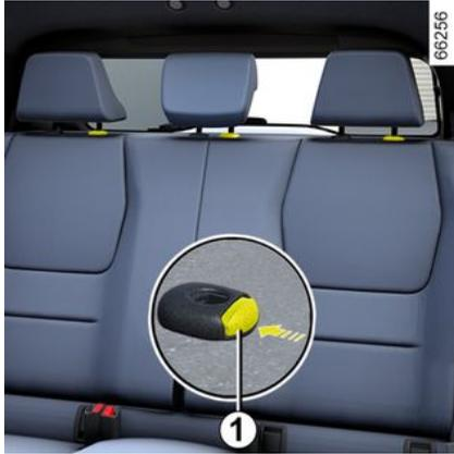
Tilt the bench seat forwards, raise the headrest as much as possible, then press button **1** and remove the headrest.
