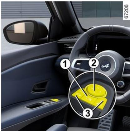
When you select a door mirror using one of the switches **3**, the indicator light built into the switch will appear. Then use the button **2** to adjust it to the desired position.
