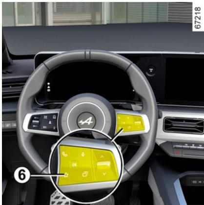
Depending on the vehicle, by pressing the steering wheel control **6** you can activate the heated steering wheel according to the stored use settings that you have previously defined.
