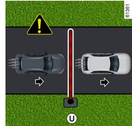
**Non-detection of fixed obstacles and objects of a small size**
