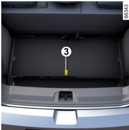
Depending on the vehicle, this tray is intended to store charging cables. The maximum permissible load per tray is 10 kg.
