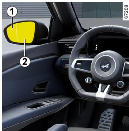
When a door is opened and a moving object is detected, the warning light **1** is displayed on the door mirror **2** and, depending on the vehicle, the ambient lights in the front door are illuminated.
