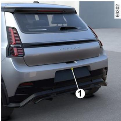
When reverse gear is engaged, the camera **1** located at the rear of the vehicle transmits a view of the area behind the vehicle to the multimedia screen **2** accompanied by three guide lines **3**, **4** or **5** (fixed, moving and trailer guide lines).
