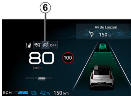
Press switch **1** as many times as necessary to select the speed limiter. The warning light **6** appears in grey. The "Speed limiter OK SET to activate" message is displayed on the instrument panel accompanied by dashes to indicate that the speed limiter function is activated and waiting for a limit speed to be stored.
