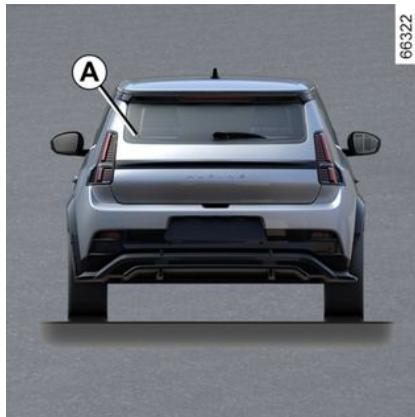
The QR Code on label **A** allows emergency workers to use a tablet or smartphone to immediately access technical information that is useful for working on the vehicle in the event of an accident.
