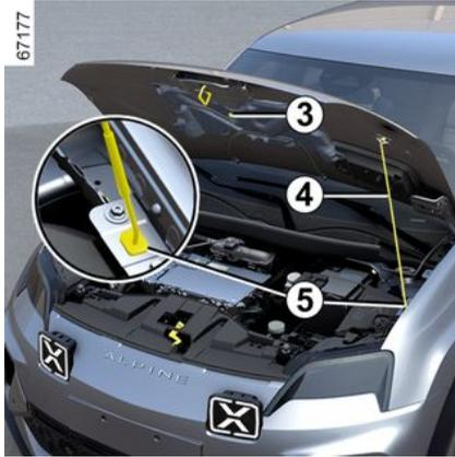
After raising the bonnet and disengaging the strut **4** from its mounting **3**, for your safety you **must** position the strut in its placement **5**.
