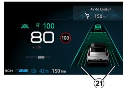
To adjust the position in the lane, the "Lane Centring" function must be in adjustment mode, the green warning light **22** must be displayed on the instrument panel and the vehicle speed must be below 31 mph (50 km/h).
