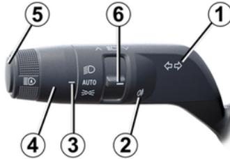
Rotate the ring **4** until the AUTO symbol is aligned with the mark **3**.
